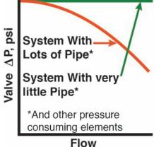
Figure 2. Valve pressure drop vs. flow
