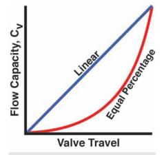
**Figure 1.** Linear and equal percentage inherent characteristics
