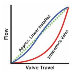
**Figure 3.** Installed characteristic of an equal percentage valve in the system with lots of pipe and other pressureconsuming elements of Figure 2
