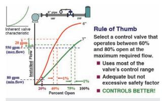
**Figure 6.** Comparison of a properly sized control valve and an oversized control valve
