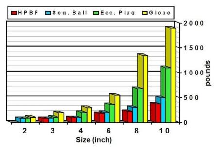
Figure 2: Control valve weight comparison
