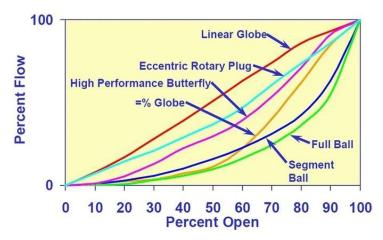
Figure 6. Typical inherent flow characteristics
