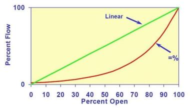
Figure 5. Ideal inherent flow characteristics
