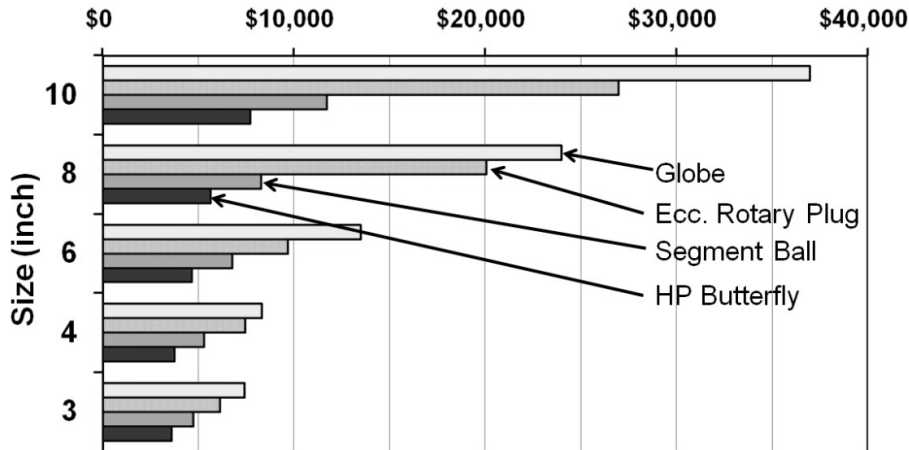
Figure 1-18. Comparison of approximate costs for High Performance butterfly valves, segment ball valves, eccentric rotary plug valves and globe valves.
