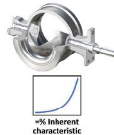
◀ Figure 2: System used in the example installed flow and gain calculations Segment valve graphic courtesy of Neles
